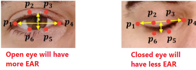
Fig. 1: Computation of Eye Aspect Ratio (EAR) from facial landmarks.
